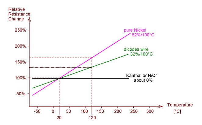
In contrast, on standard mods without temperature control, the wire is chosen to have no or very little temperature dependency, like Kanthal or NiCr.
